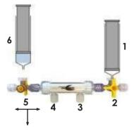
Detach the syringe containing the recovered particles from the nozzle 6 and collect into a clean tube.
