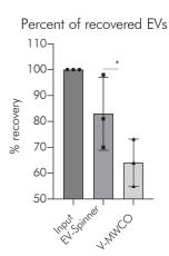
FIG 2. EV-Spinner allowed consecutive concentrations (from 2.5 ml up to 0.25 ml) with minimun clogging of the filter. The clogging of the filter was measured by the time necessary for concetrating a solution of EVs from 2.5 ml up to 0.25 ml.
