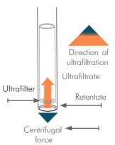
After centrifugation, remove the inner tube with the tweezers supplied. Recover the concentrated sample (retentate) in the outer tube with a micropipette.
