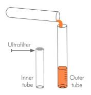
Re-insert the inner tube with the membrane side first. Ensure the membrane is in contact with the sample. Do not re-insert the cap for centrifugation.
